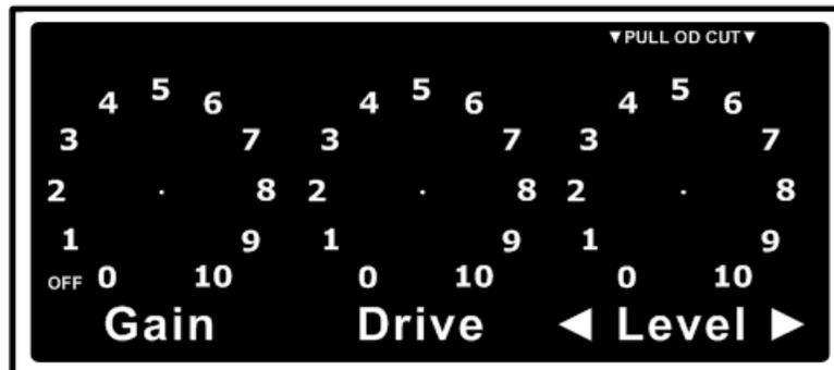
The Drive section controls the amount of character to add to the Blackface channel's tone. The section's range of effect can be just a hint of early break up or a full on aggressive heavy metal distortion.
