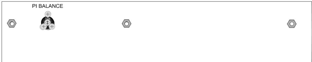
The BTS2 has 1 internal trim pot for the PI Balance – Useful for working with unmatched 12AX7 tubes in the phase inverter position. Refer to qualified personnel for proper setting.
