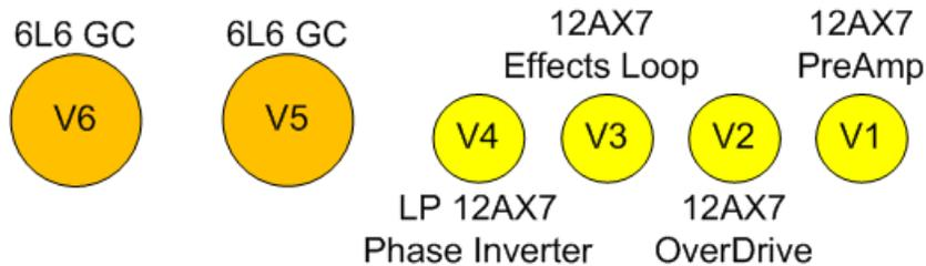
All tube brands are acceptable, a long plate is preferred in the V4 (Phase Inverter) position. The Overdrive tube is also the Tweed preamp tube. 6V6GTA can be substituted for the 6L6 GC tubes for less wattage but do not mix the 2 types.
