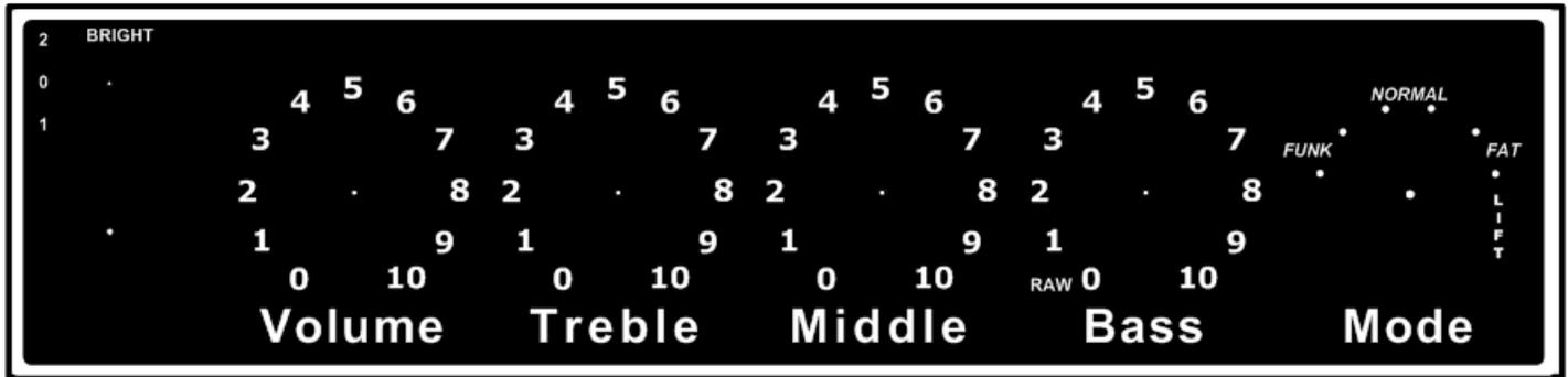
The Clean Preamp is designed to imitate (and surpass) all of the “classic” guitar amp preamps. The BTS2 Mode control gives the player the ability to shift midrange center point frequency.
