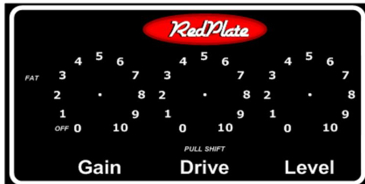
The Drive section controls the amount of character to add to the clean tone. The section's range of effect can be just a hint of early break up or a full on aggressive heavy metal distortion.
