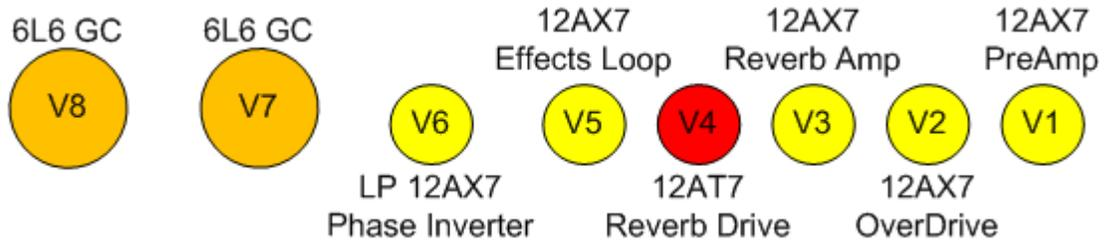
All tube brands are acceptable, a long plate is preferred in the V6 (Phase Inverter) position.
