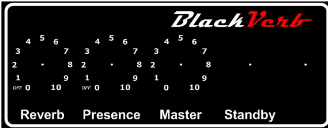
**Reverb Control** - Sets the amount of reverberation effect, takes the reverb out of circuit when rotated to zero (there will be a slight volume and tone change).
